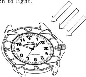
1. Expose the watch to sunlight or strong artificial light of more than 1,000 lux (for example, two 15-watt fluorescent lights with a distance of 70 cm between the watch and the light source). It will start operating immediately with the second hand moving at 2-second intervals.
