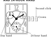
Pull out the crown all the way to the second click when the second hand is at the 12 o'clock position. The second hand will stop on the spot. o'clo stop
