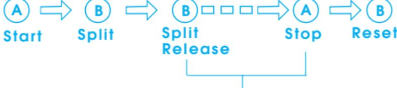
\* Measurement and release of split time can be repeated by pressing button "B".
