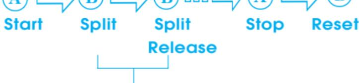
\* Measurement and release of split time can be repeated by pressing button B.
