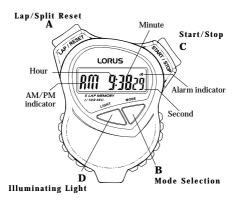
Press button B to select display mode. Display mode changes over in the following order by each press of the button.
