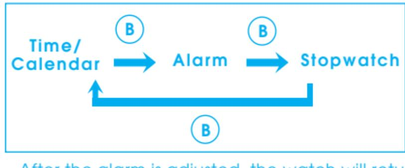
\* After the alarm is adjusted, the watch will return to the Time/Calendar display when button B is pressed.
