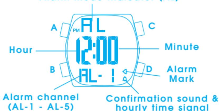
1. Press button B in the Time/Calendar or Dual Time display to go to the Alarm mode. Mode indicator "AL" appears.
