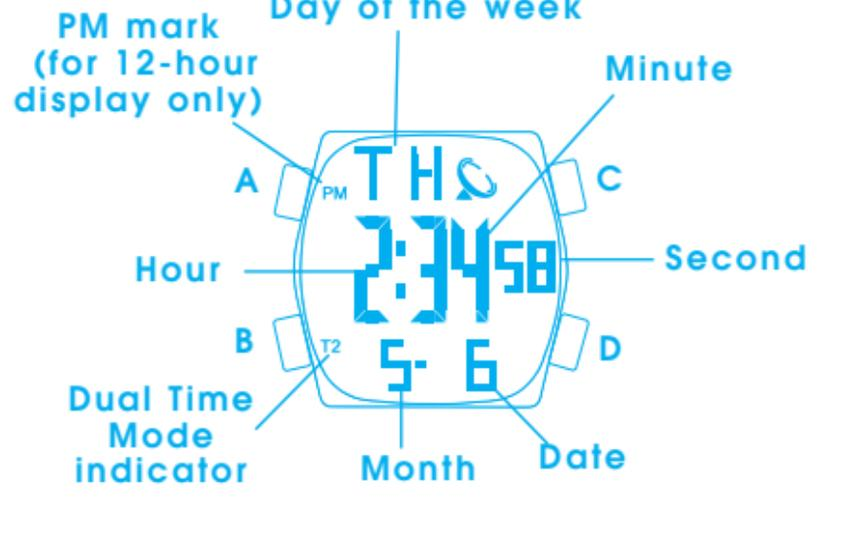
1. Press button C in the Time/Calendar display to go to the Dual Time mode. Mode indicator "T2" appears.
