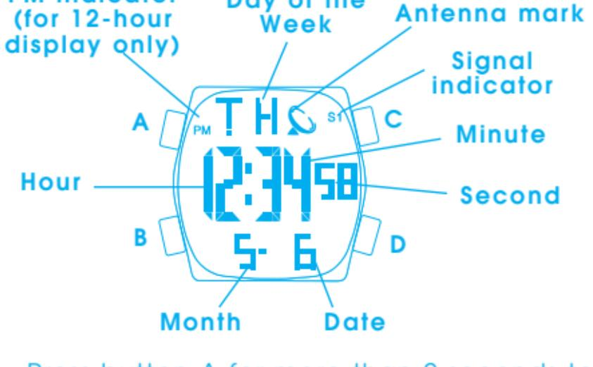
1. Press button A for more than 2 seconds to go to the Time/Calendar Setting Mode. The signal selection digit starts flashing.
